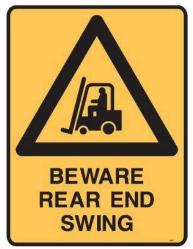
Operators need to keep to the inside of every turn to allow enough room for the rear of the forklift to swing around.
